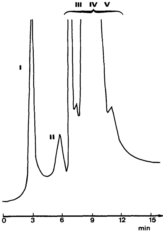
Figure 4.- HPLC separation of the proteins from fraction a obtained using Sephadex G-100 gel-filtration. Fraction a (50 \mu l collected at the top of the fraction) was loaded on a Waters column ; elution with EP 2 ; flow rate, 1.5 ml/min ; detection at 215 nm (0.01 AUFS) ; chart speed, 1 cm/min.
